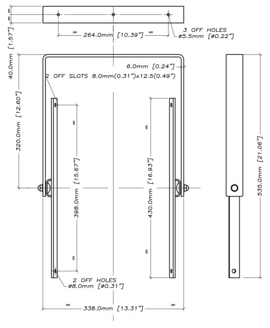
SUPPLIED HARDWARE:4 OFF M8×40mm CAP HEAD SOCKET SCREWS
